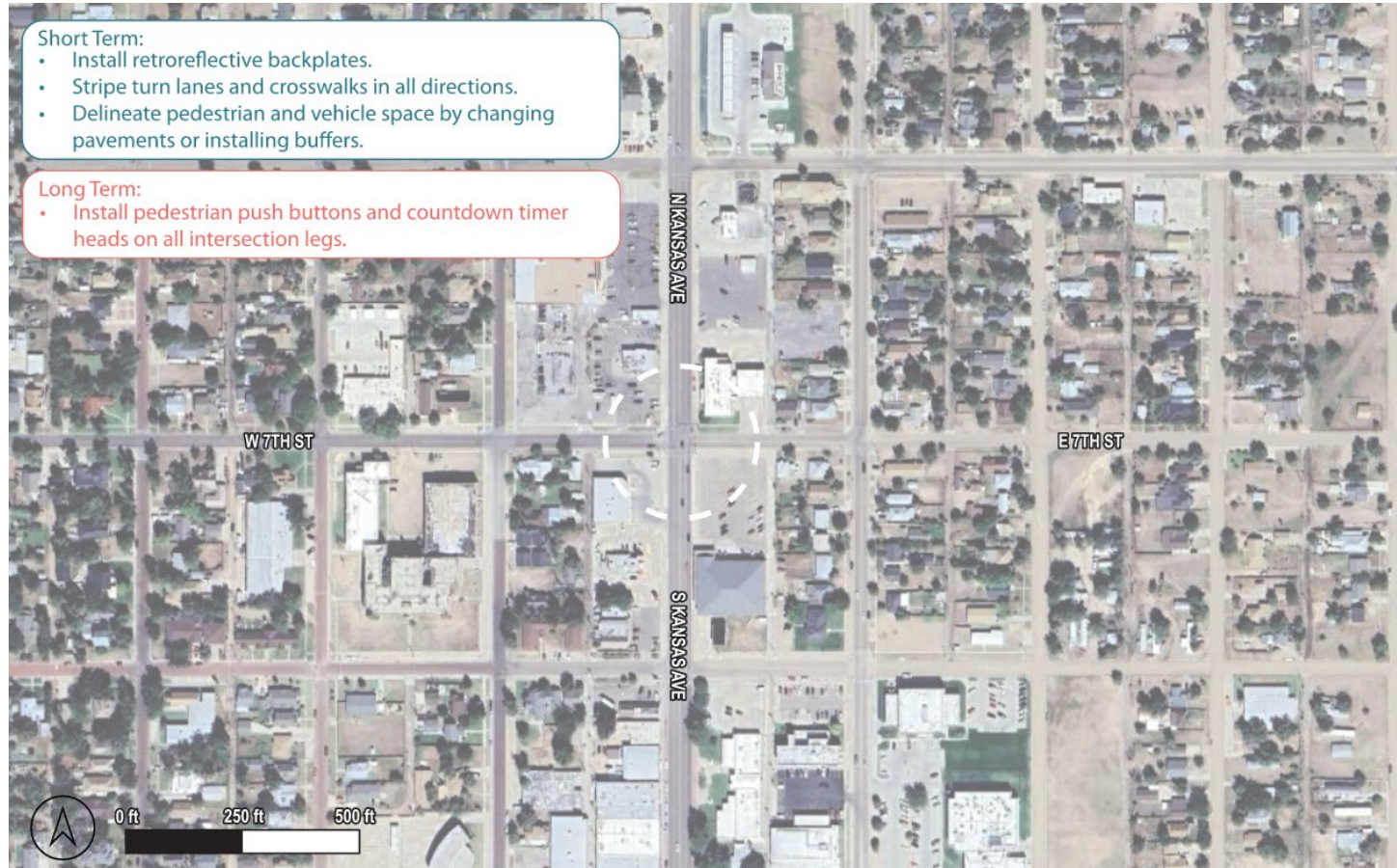
Figure 35: Intersection of Kansas Ave and 7 th St (Project 58)
