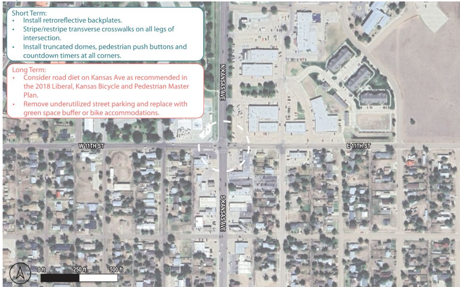
Figure 36: Intersection of Kansas Ave and 11 th St (Project 59)
