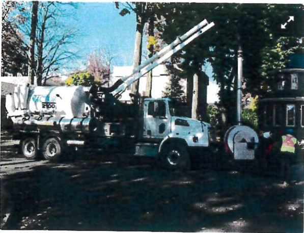
A combination sewer cleaner with a positive-displacement configuration is ideal for pulling material long distances and tackling the deep pulls.
